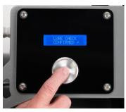
The display will then change to "set pressure". A default pressure of 100BAR (1450PSI/10MPa) is displayed.
